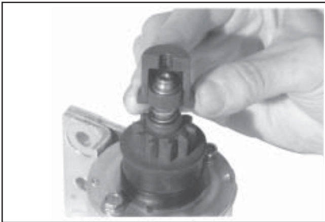
Figure 8-38. Assembling Larger Inner Half Around Spring Retainer.
